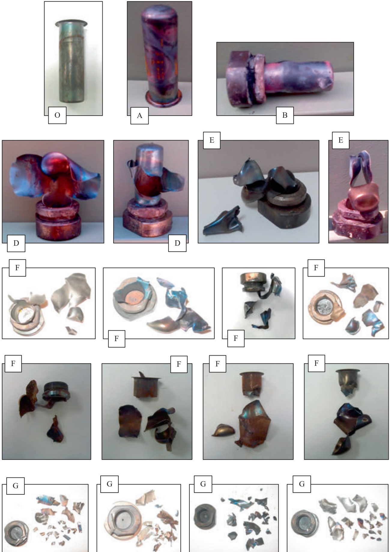
Figure 18.6.1.4: Examples of Koenen test results
