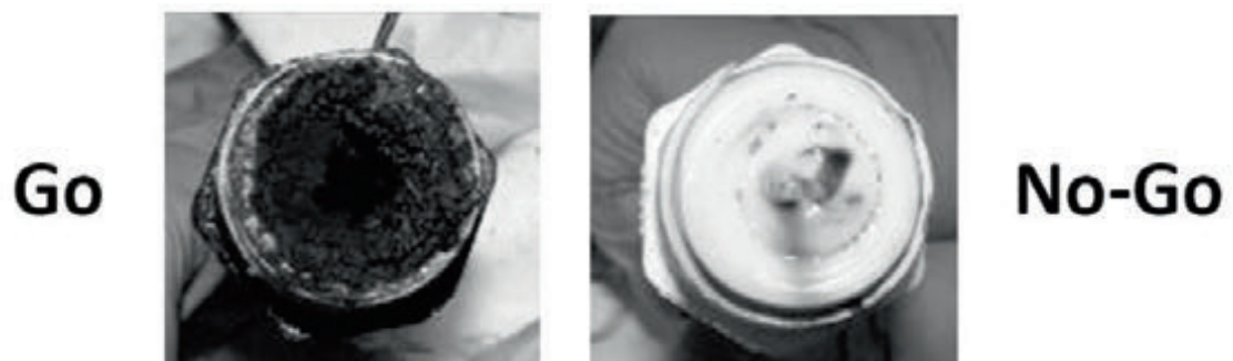
Figure 18.8.3: Typical aspect of the test cell after a "go" (left) and "no-go" (right) event
