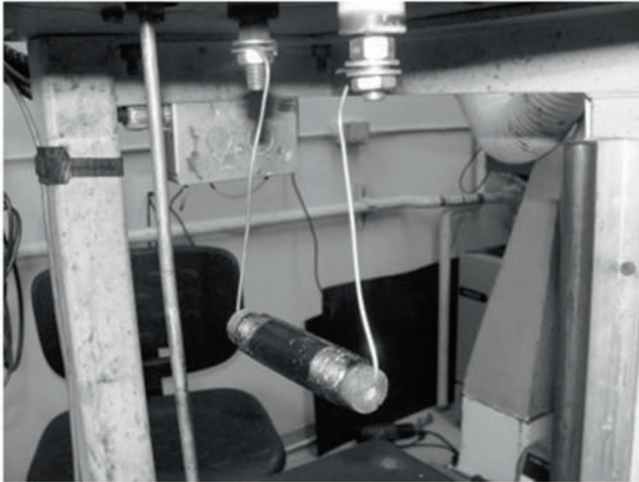
Figure 18.8.2: Test cell mounted horizontally under the cover of the pressure vessel (copper conductors connected to vessel's fixed electrodes)
